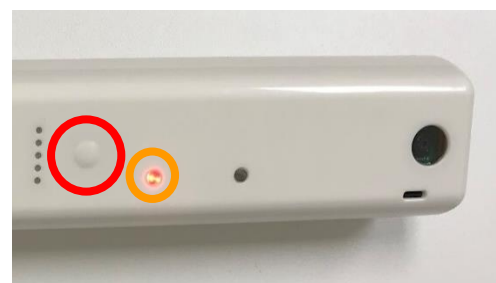
Figure 1.2 – Front Panel Indicators
